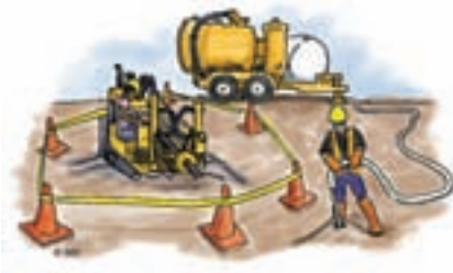
Vakumlu Kazı Vacuum Excavator
